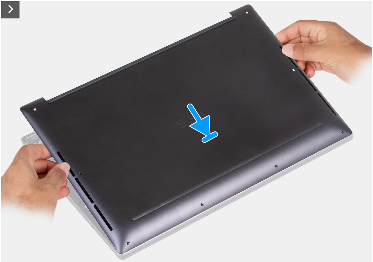
Figure 13. Placing the base cover into slots on the palm-rest assembly
