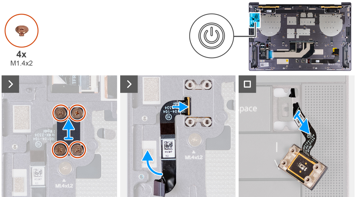
Figure 37. Removing the power button with fingerprint reader
