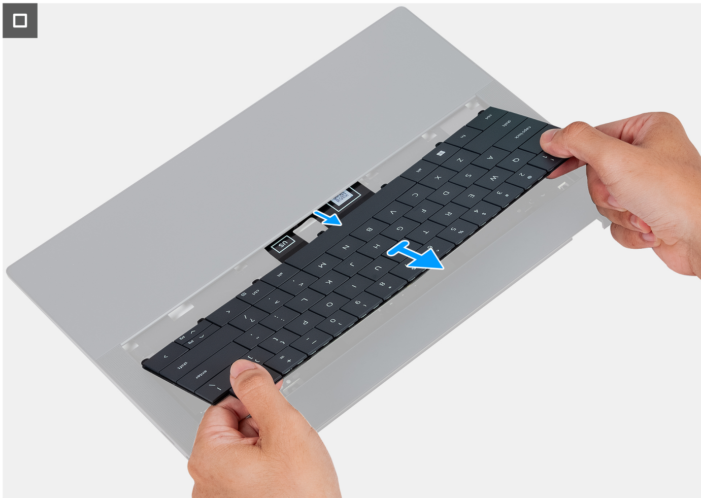
Figure 41. Removing the keyboard
