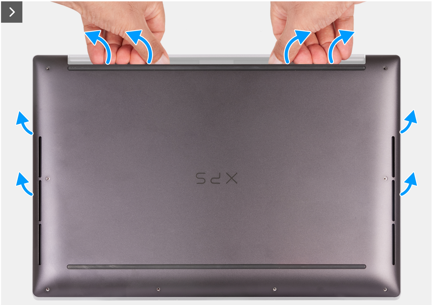
Figure 9. Using both thumbs to pry the base cover
