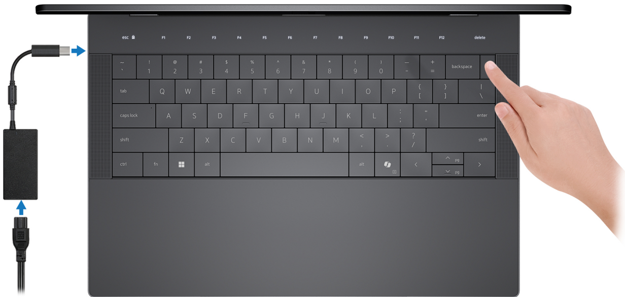
Figure 7. Connect the power adapter and press the power button.
