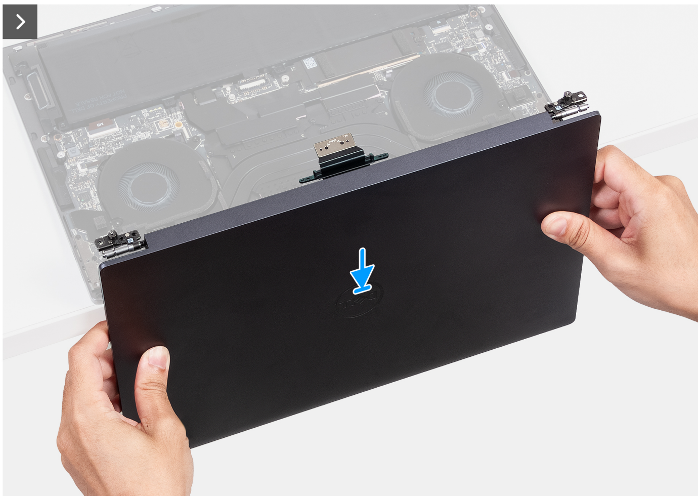
Figure 29. Installing the display assembly
