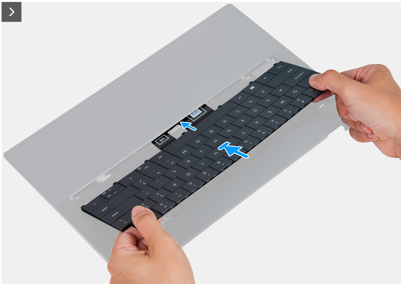
Figure 42. Installing the keyboard
