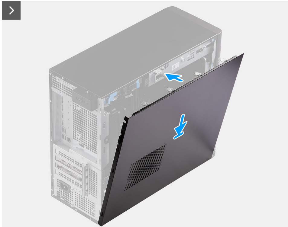
Figure 10. Installing the side cover
