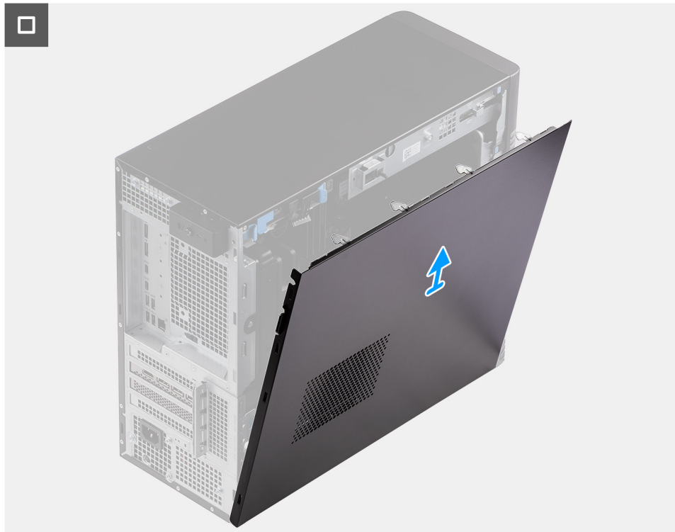
Figure 9. Removing the side cover
