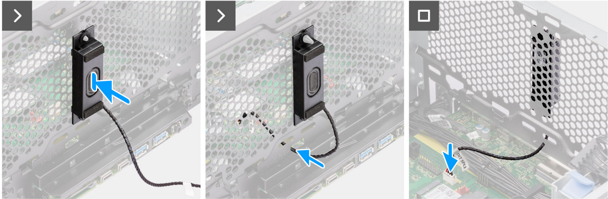
Figure 73. Installing the internal speaker
