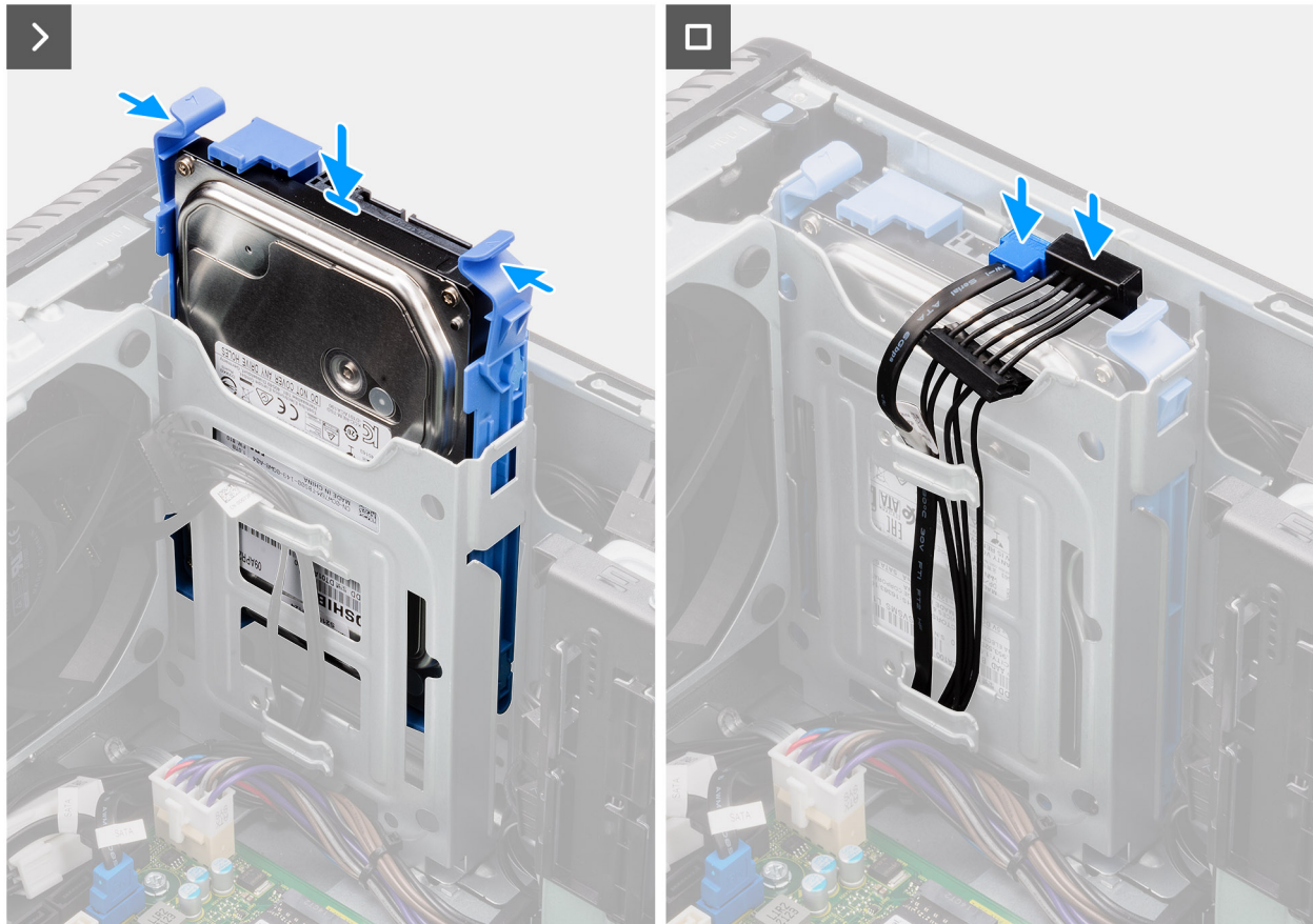
Figure 21. Installing the 3.5-inch hard drive assembly from Bay 1
