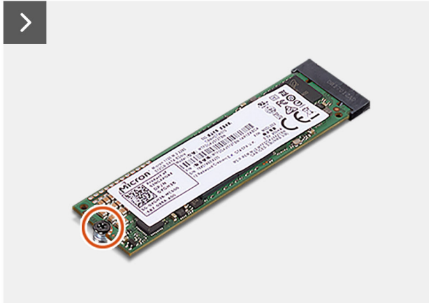
Figure 24. Removing the M.2 2280 PCIe solid state drive
