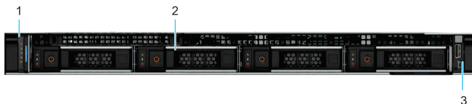
Figure 1. Front view of 4 x 3.5-inch drive system
