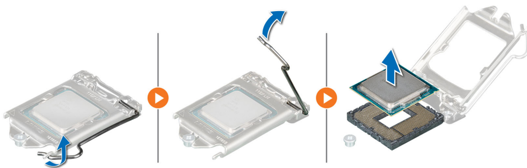
Figure 45. Removing the processor
