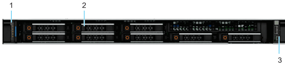
Figure 2. Front view of 8 x 2.5-inch drive system
