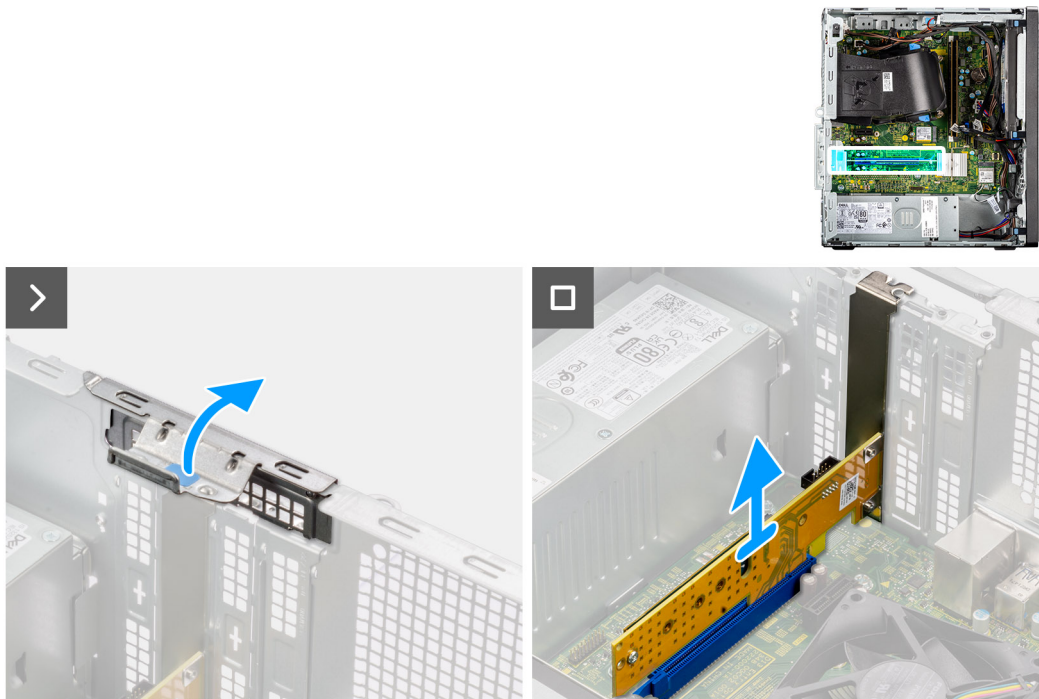
Figure 25. Removing the Dell Ultra Speed Drive Gen3 card
