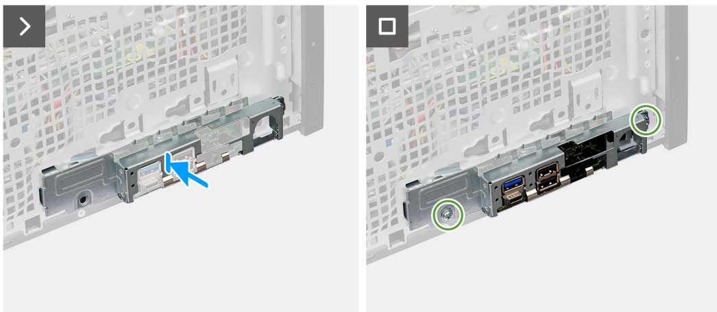
Figure 91. Installing the system board
