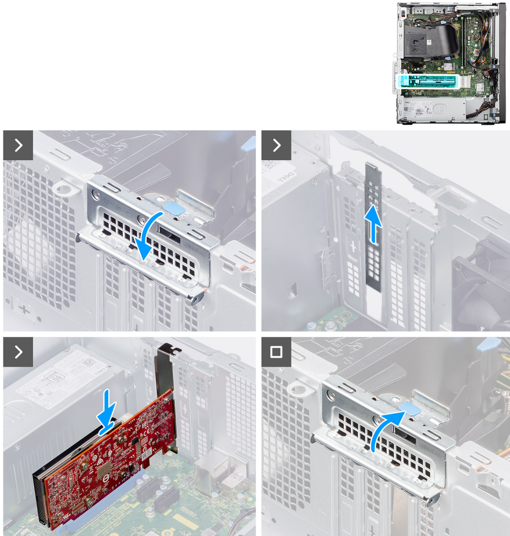
Figure 34. Installing the graphics card
