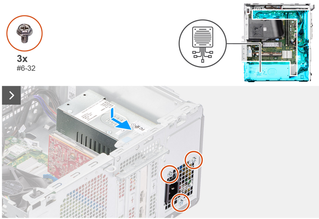
Figure 66. Installing the power-supply unit
