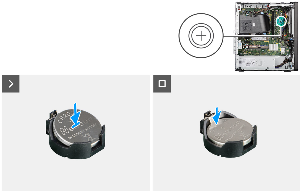
Figure 14. Installing the coin-cell battery
