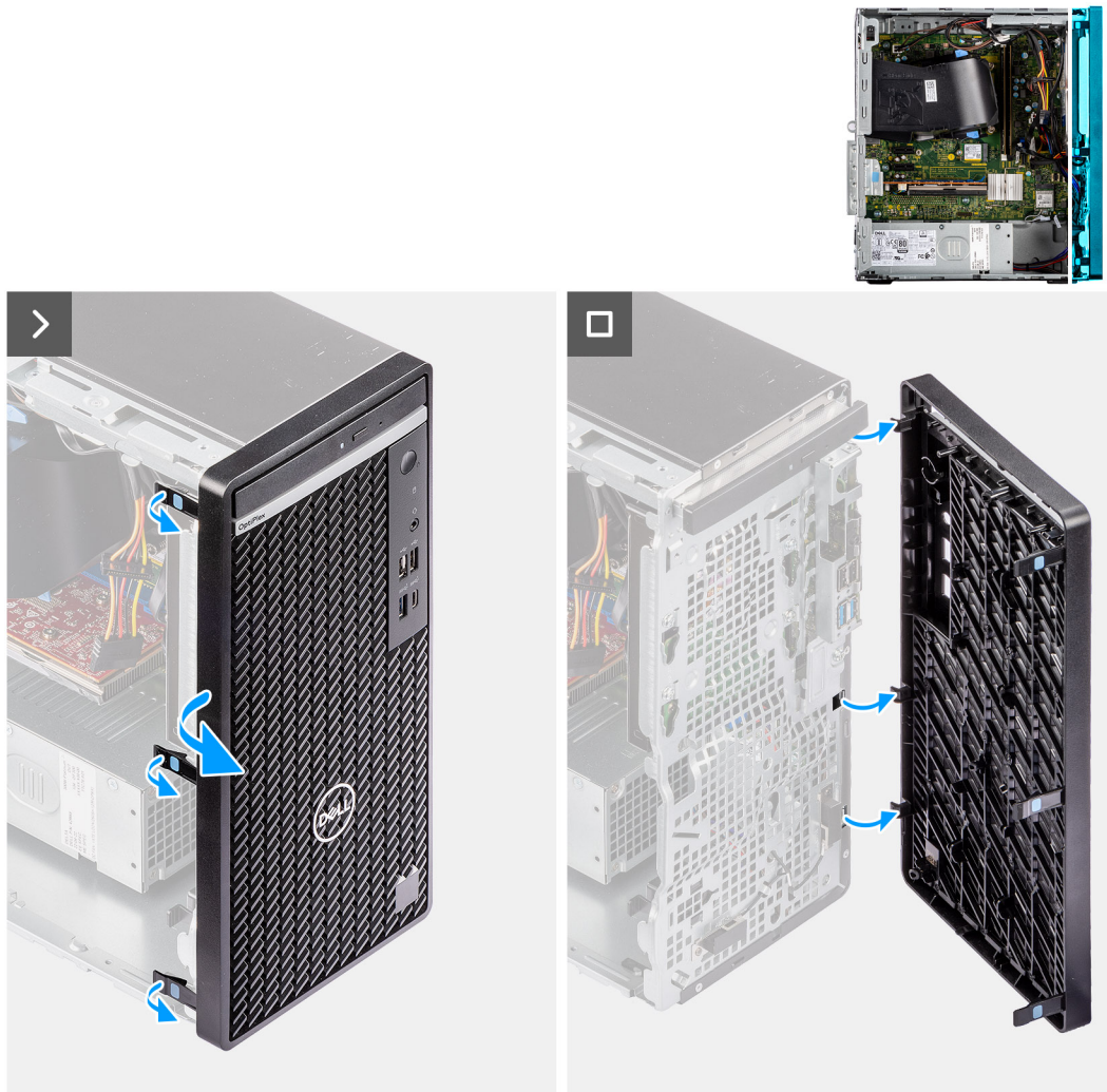
Figure 15. Removing the front bezel
