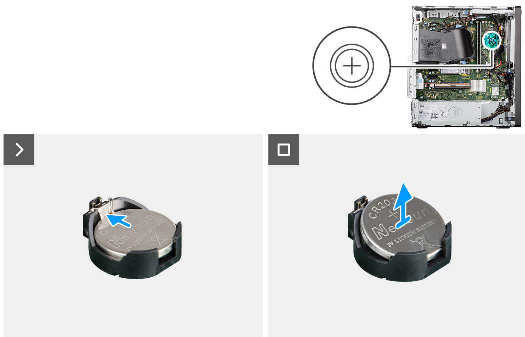
Figure 13. Removing the coin-cell battery
