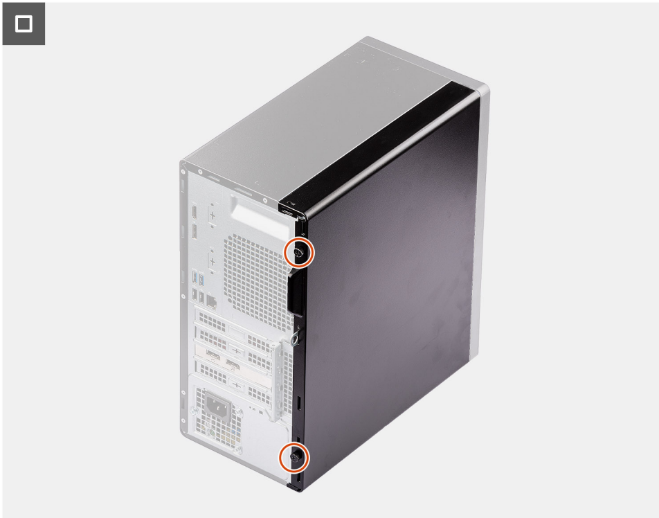
Figure 12. Installing the side cover
