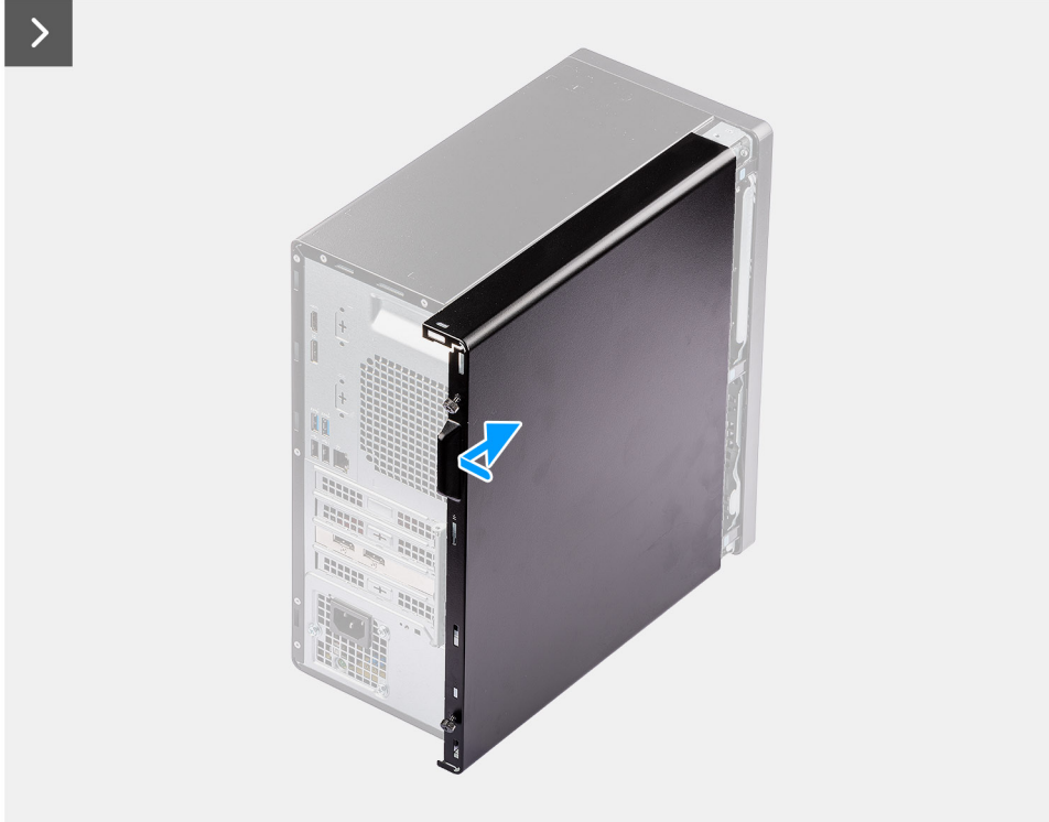
Figure 11. Installing the side cover
