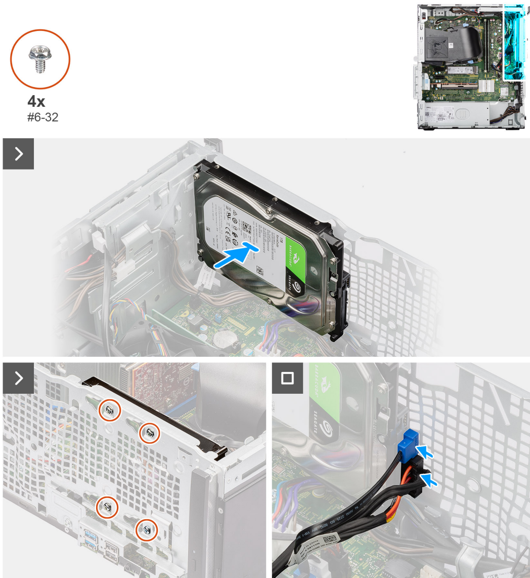
Figure 36. Installing the 3.5-inch hard drive
