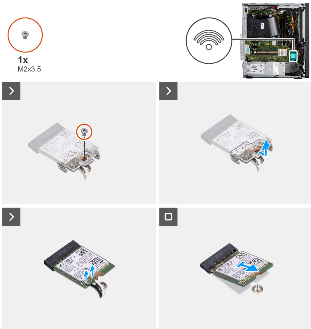
Figure 31. Removing the wireless card
