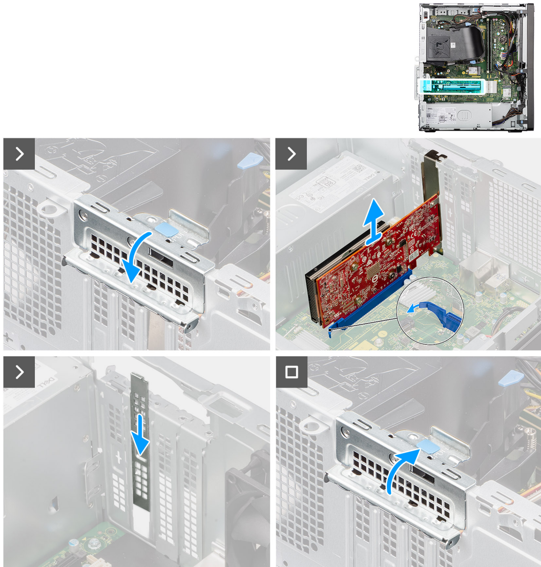
Figure 33. Removing the graphics card
