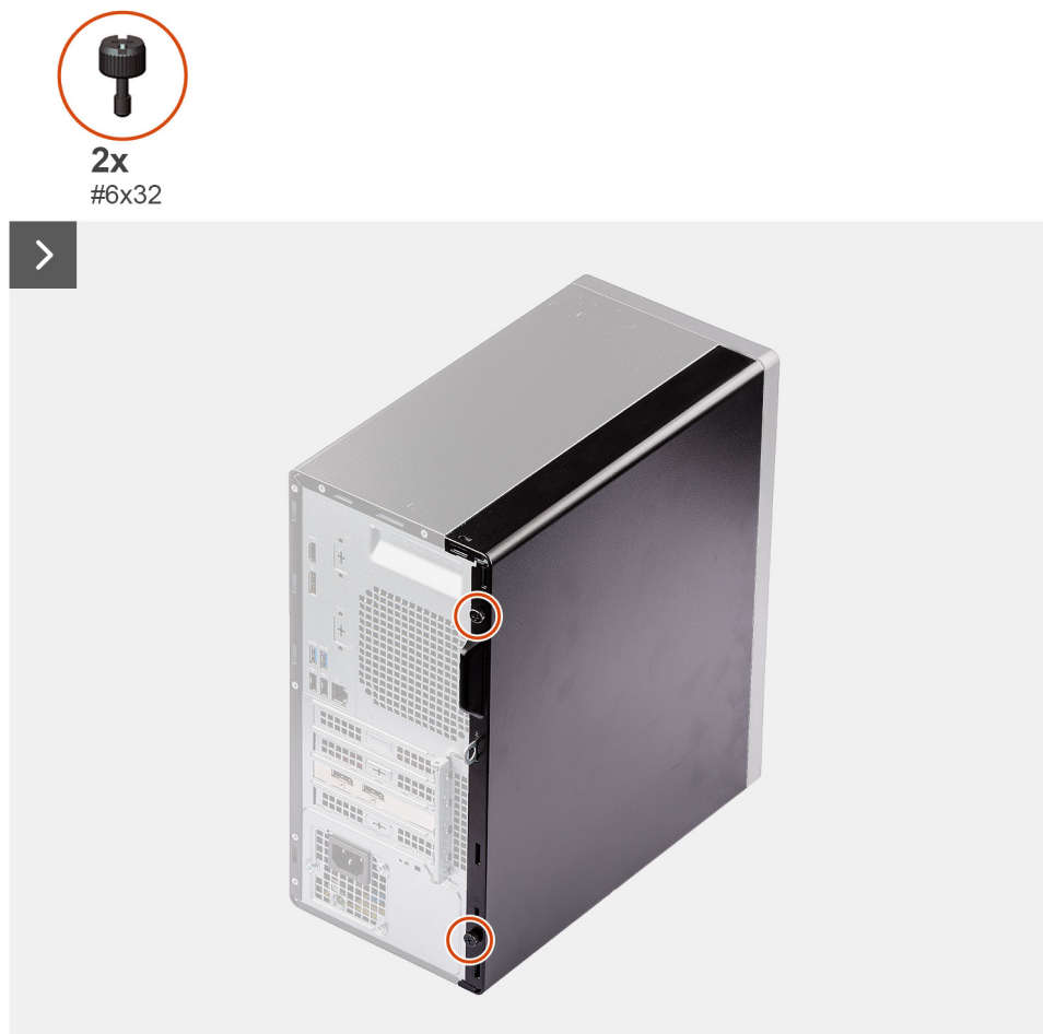
Figure 9. Removing the side cover
