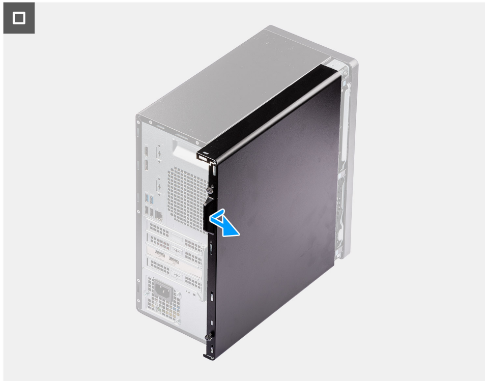
Figure 10. Removing the side cover
