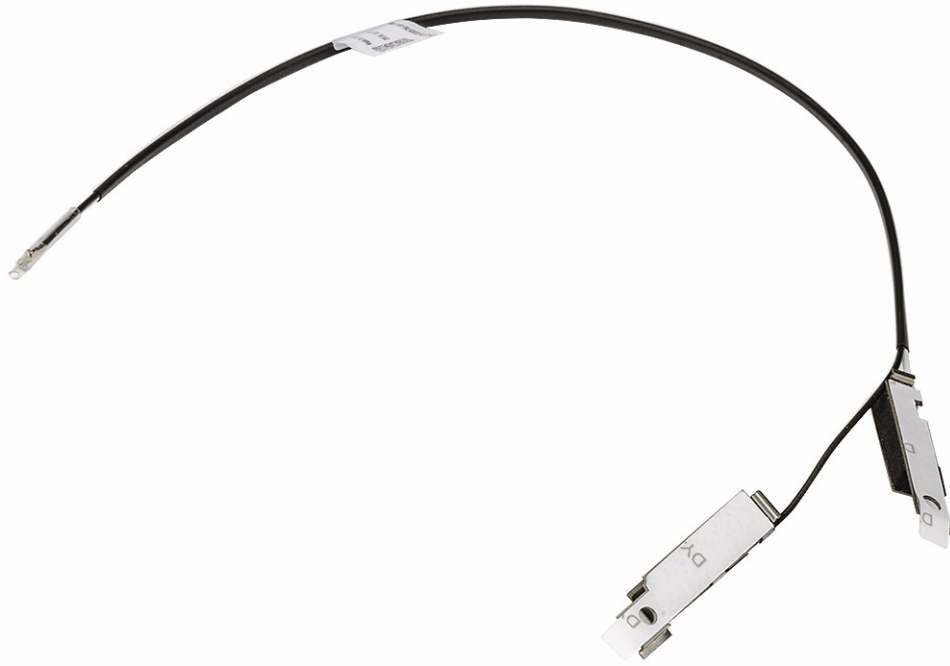
Figure 38. Internal antenna module
