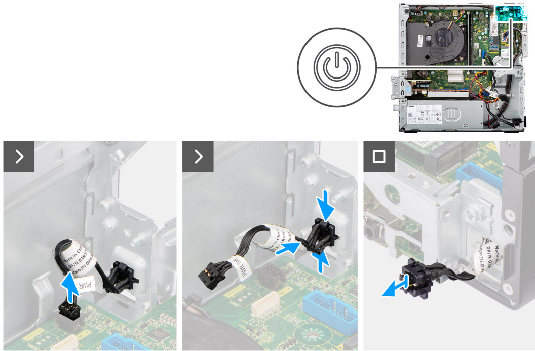
Figure 35. Removing the power button
