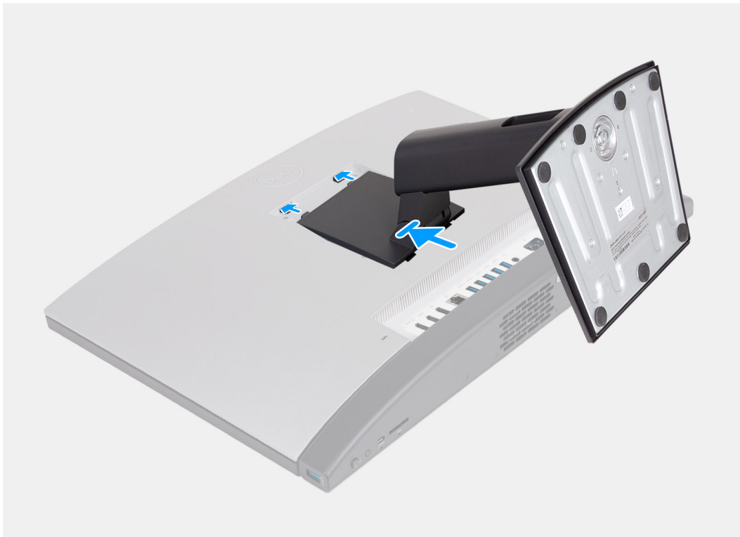
Figure 21. Installing the Fixed Stand
