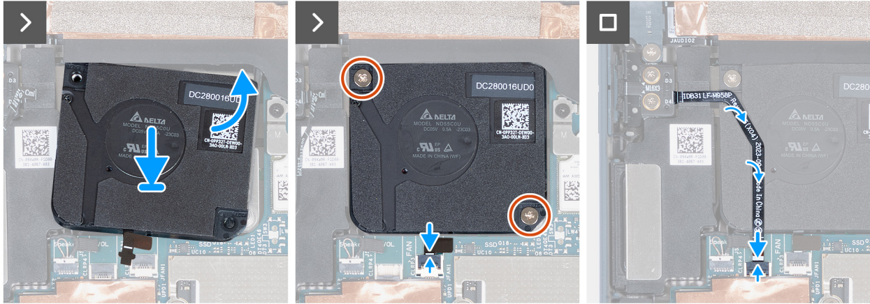
Figure 36. Installing the left fan
