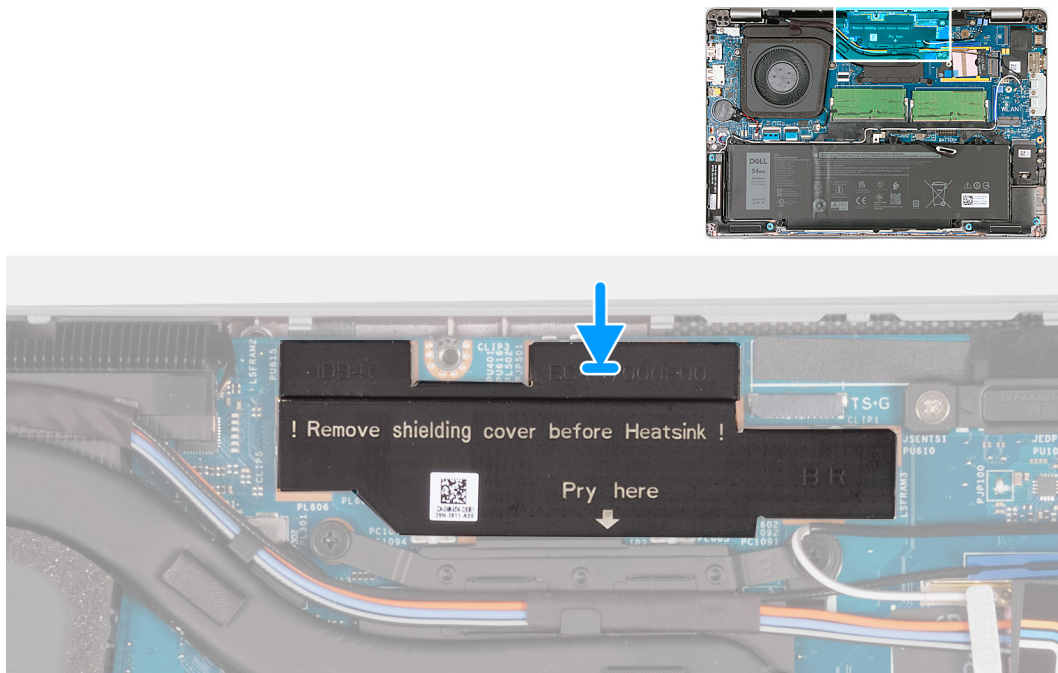
Figure 35. Installing the power shielding cover - For computers shipped with H28 UMA system board
