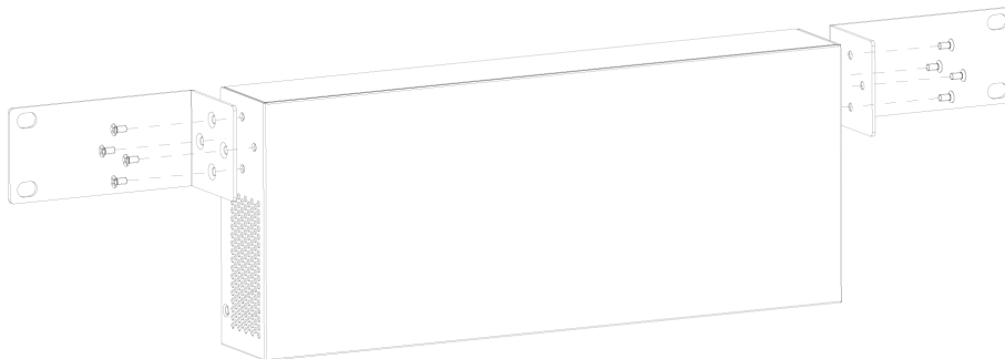
Figure 3-1 L-shaped bracket installation
