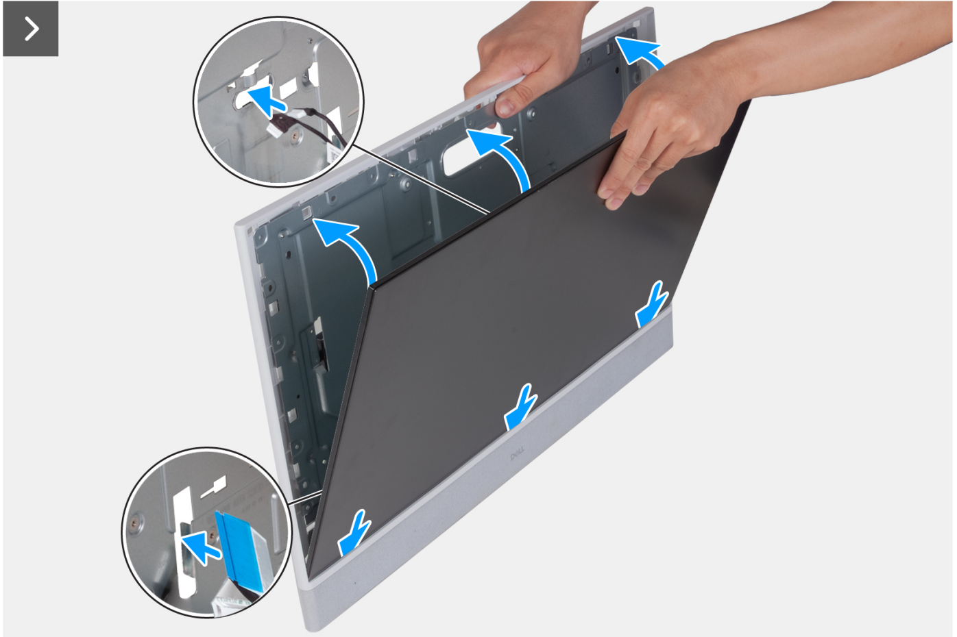
Figure 62. Installing the display panel
