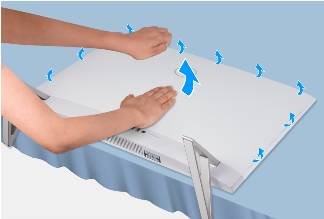
Figure 20. Removing back cover
