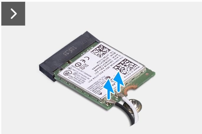
Figure 32. Removing the wireless card
