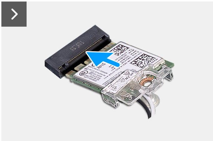
Figure 33. Installing the wireless card
