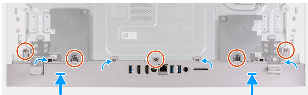
Figure 23. Installing bottom cover
