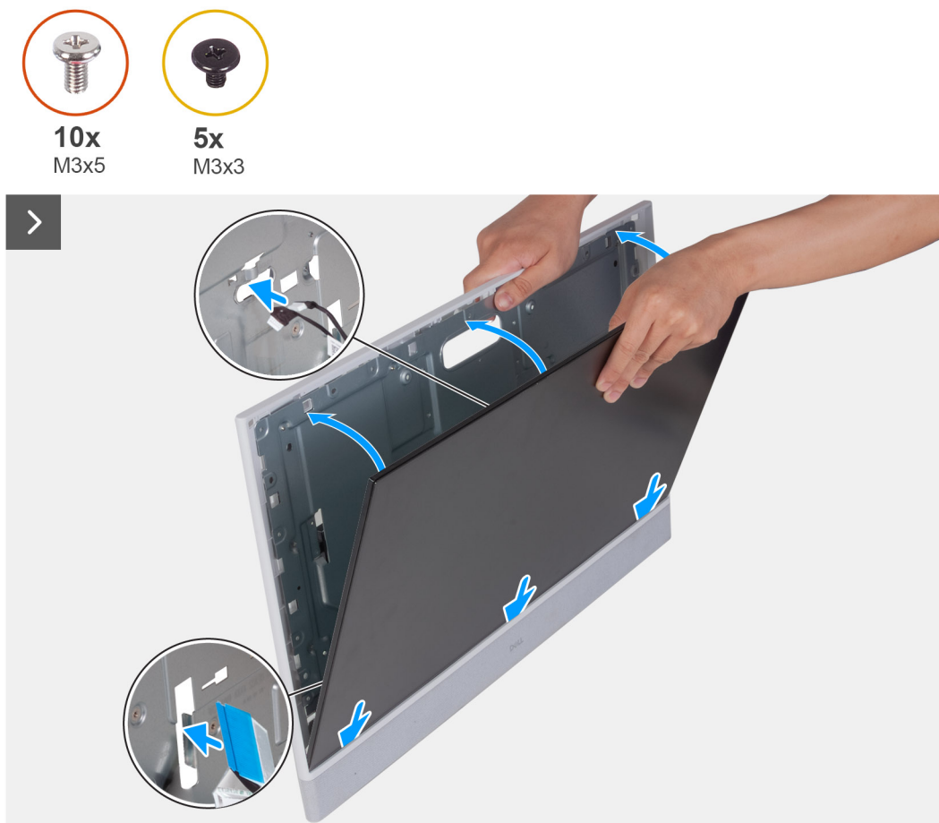
Figure 62. Installing the display panel
