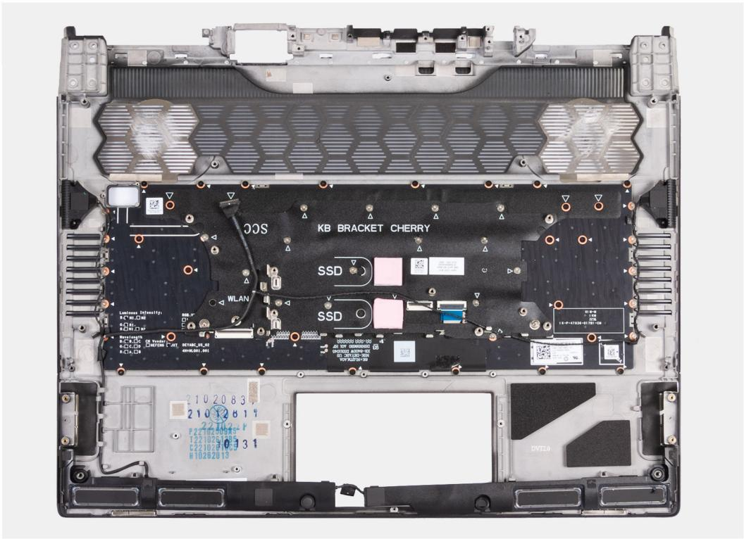
**Figure 84. Removing the palm-rest and keyboard assembly**
