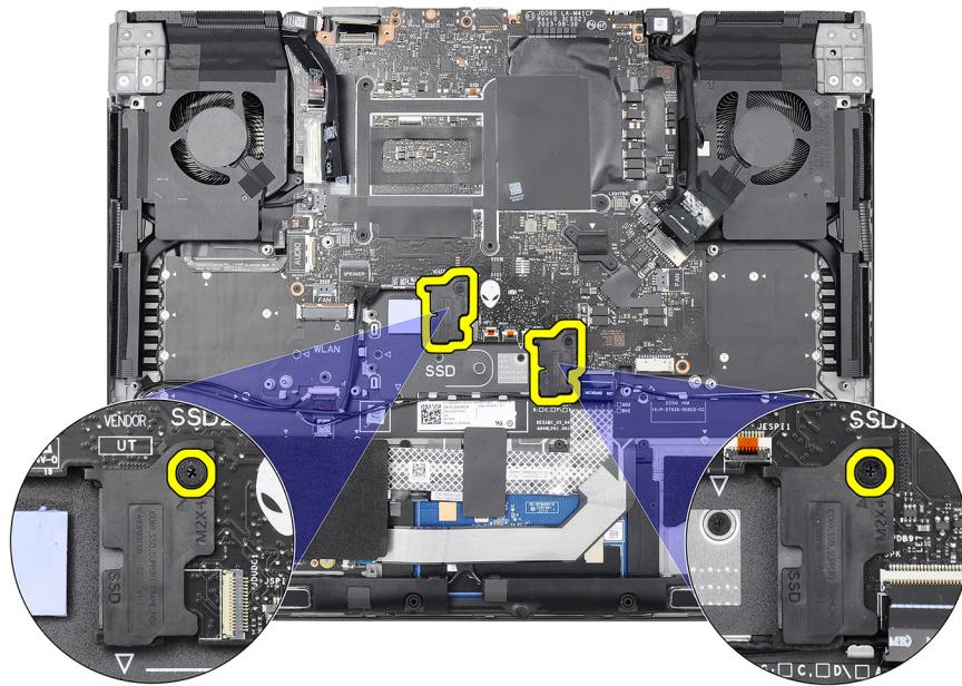
**Figure 20. Solid state drive bracket**
