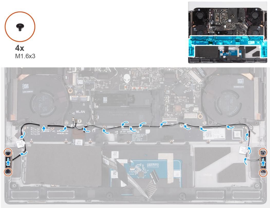
**Figure 59. Installing the antennas**
