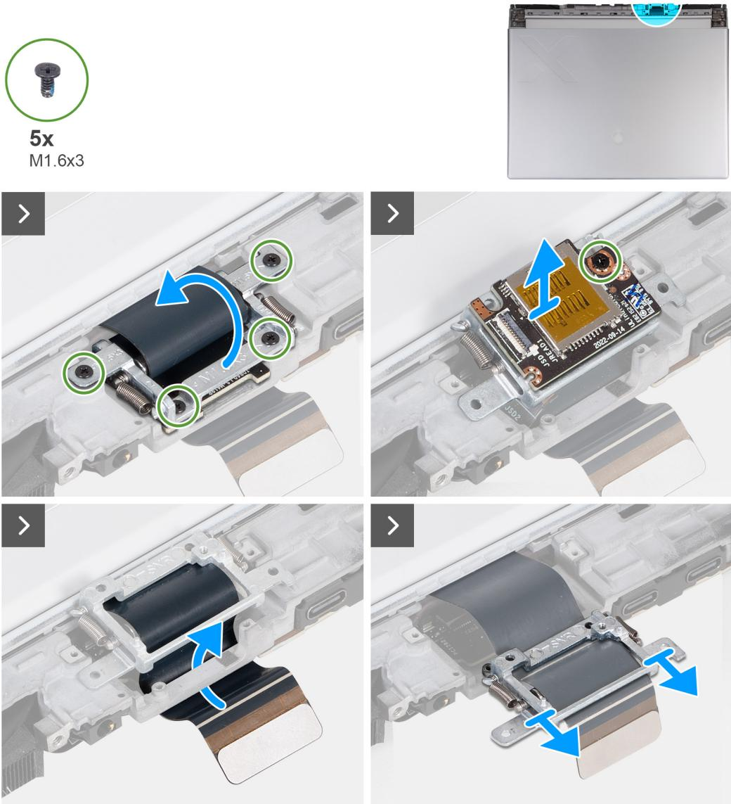
**Figure 51. Removing the display assembly**
