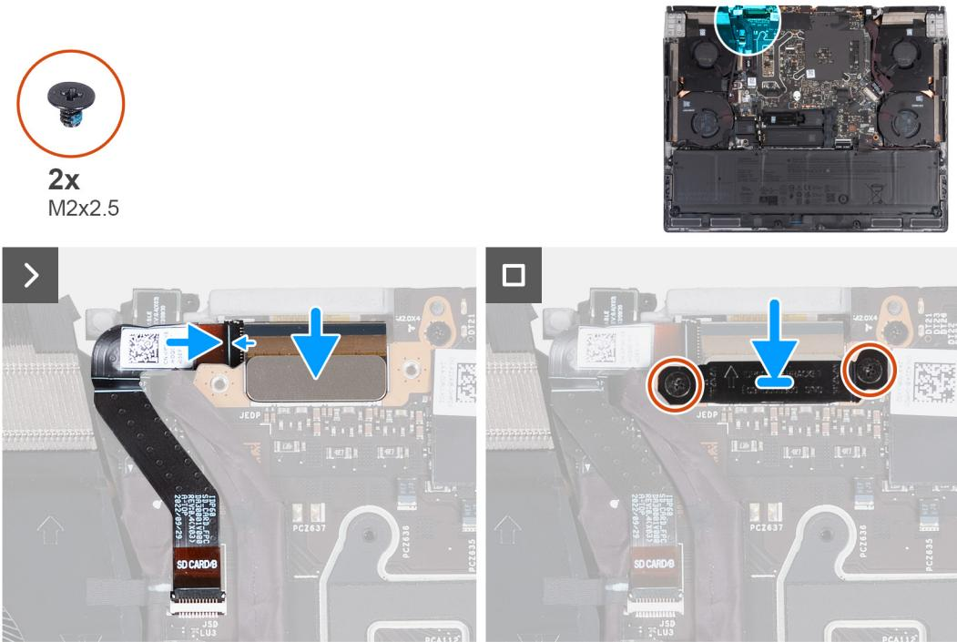
**Figure 47. Installing the microSD-card reader**
