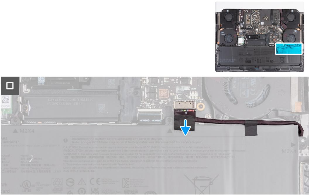
**Figure 11. Disconnecting the battery cable**
