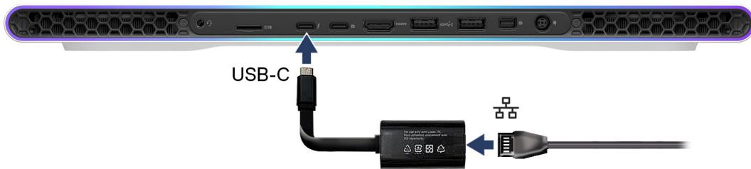
**Figure 7. Connect the USB Type-C Ethernet dongle**
