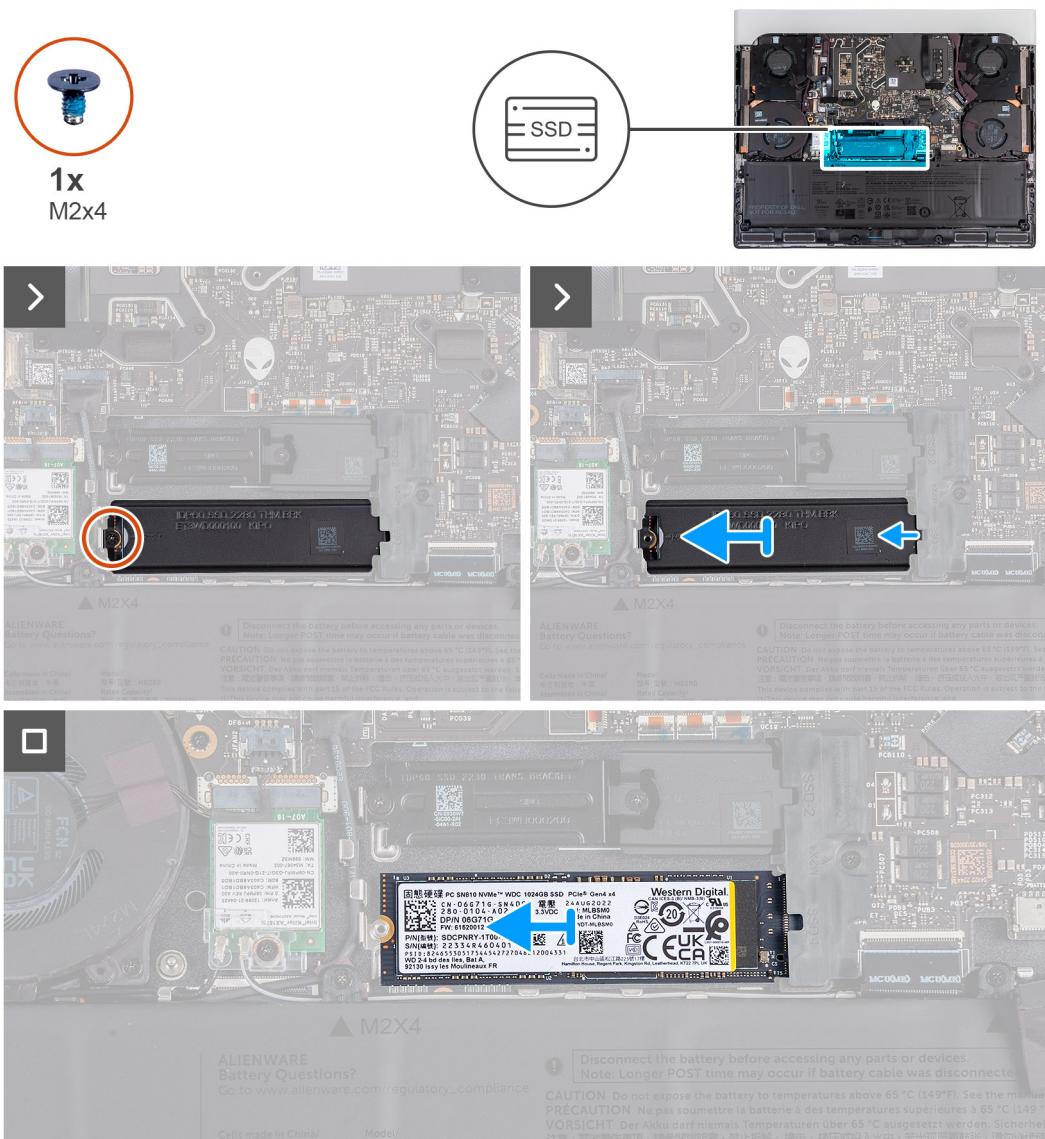
**Figure 17. Removing M.2 2280 SSD in SSD-1**
