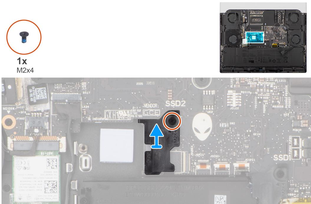
**Figure 19. Removing the solid state drive bracket**
