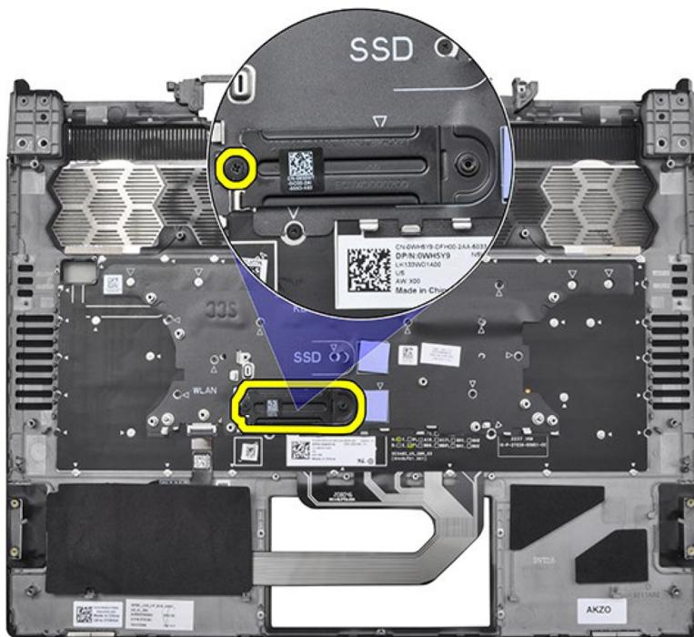
**Figure 85. Removing the palm-rest and keyboard assembly**
