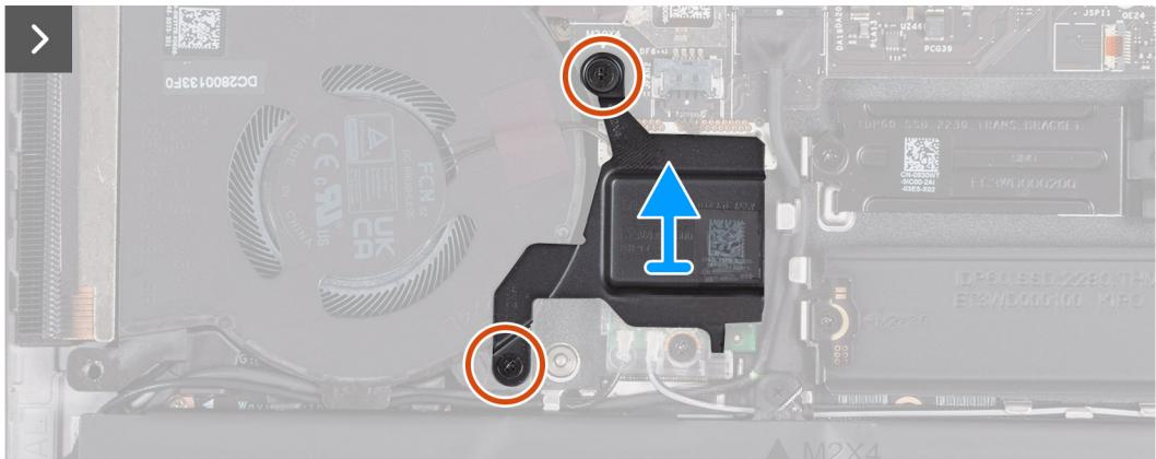
**Figure 25. Removing the wireless card thermal shield**
