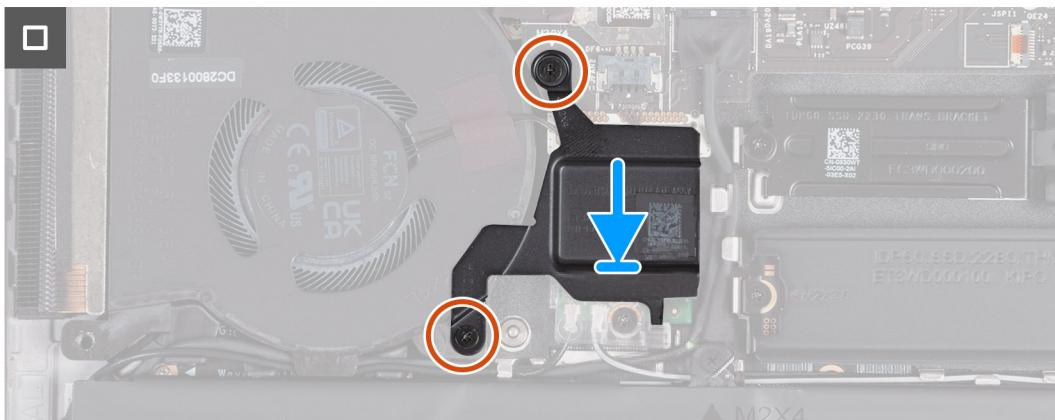
**Figure 28. Installing the wireless card thermal shield**
