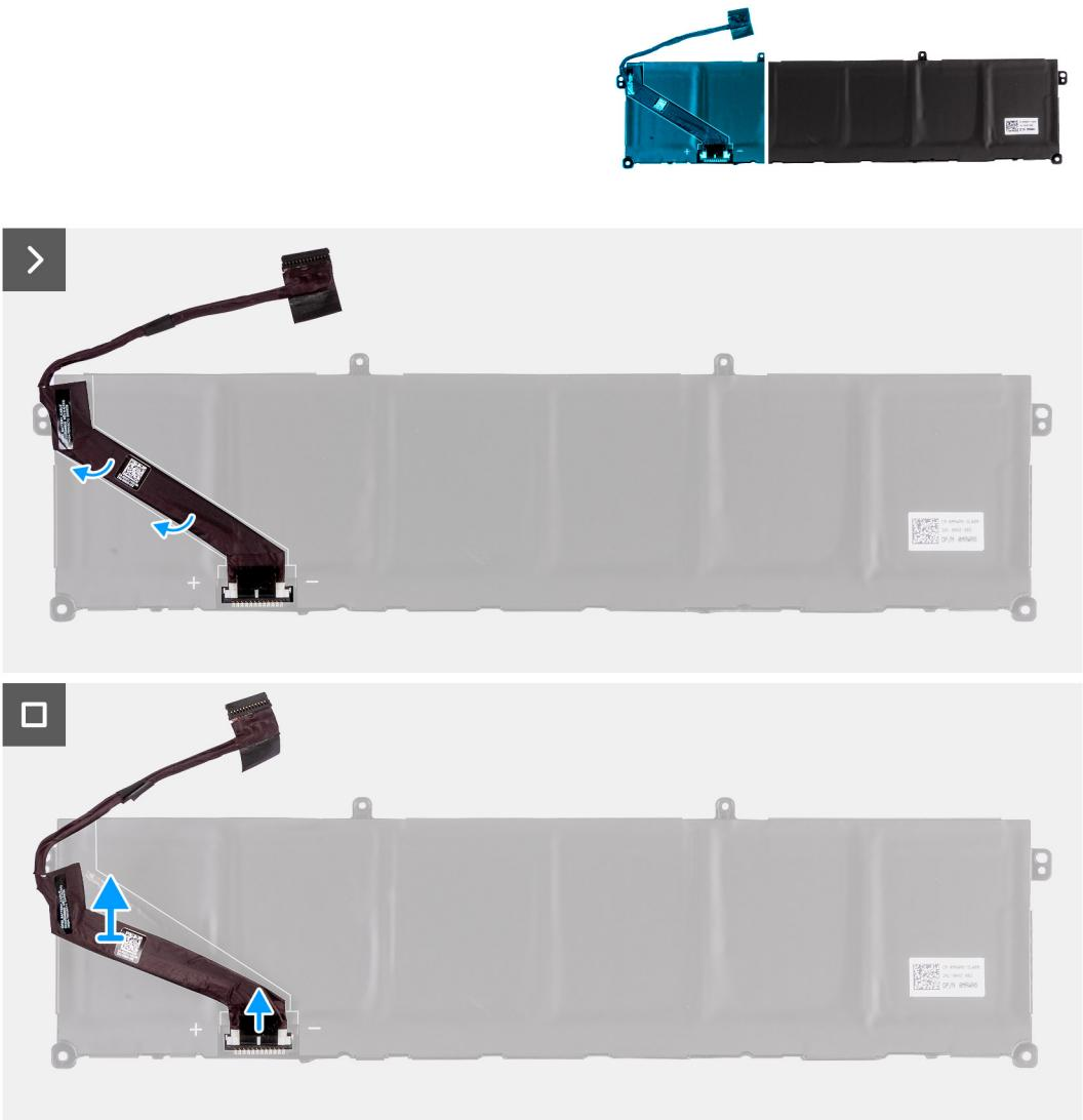
**Figure 33. Removing the battery cable**
