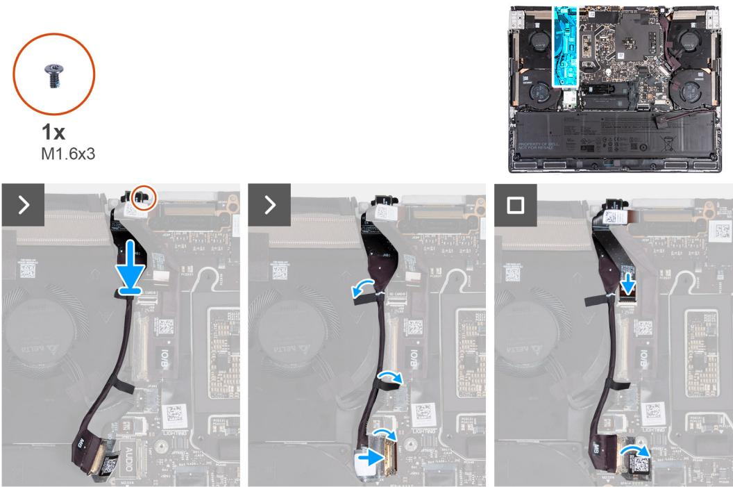
**Figure 43. Installing the headset port**
