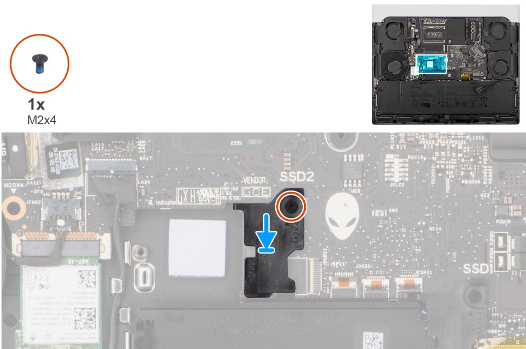
**Figure 22. Installing the solid state drive bracket**
