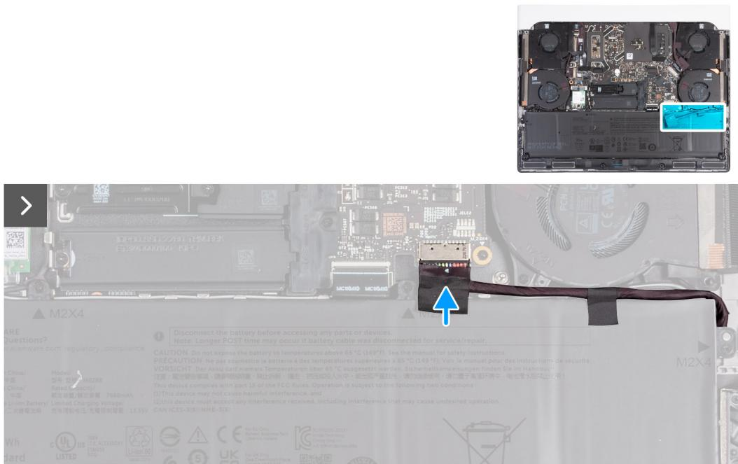
**Figure 12. Connecting the battery cable**
