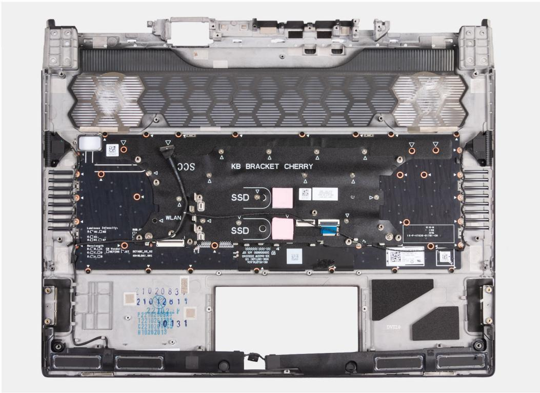
**Figure 88. Installing the palm-rest and keyboard assembly**
