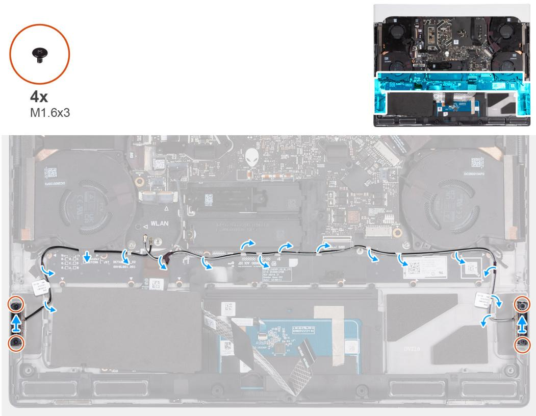
**Figure 58. Removing the antennas**
