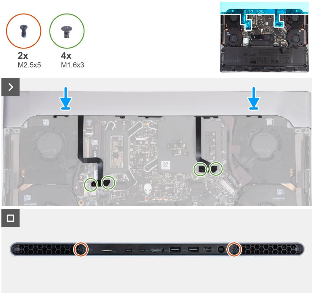
**Figure 30. Installing the rear I/O cover**
