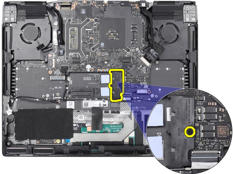
**Figure 21. Solid state drive bracket**
