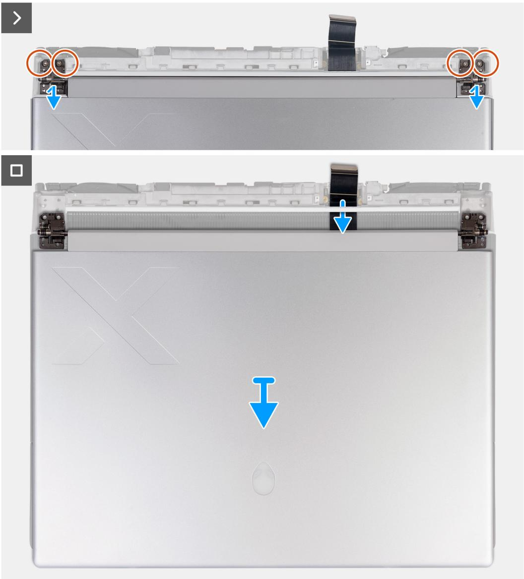
**Figure 52. Removing the display assembly**
