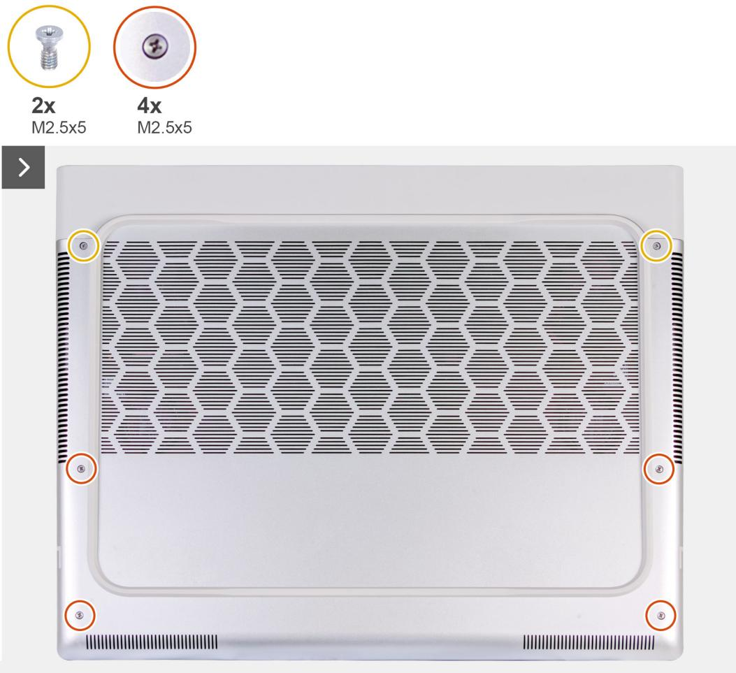
**Figure 9. Loosen the captive screws**
