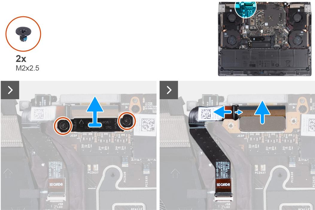
**Figure 44.** Removing the microSD-card reader
