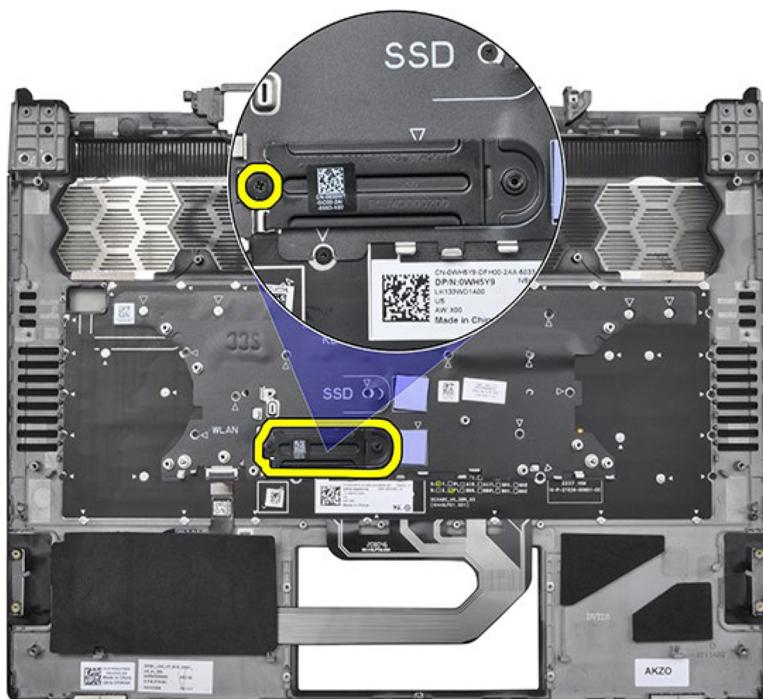
**Figure 86. Installing the palm-rest and keyboard assembly**
