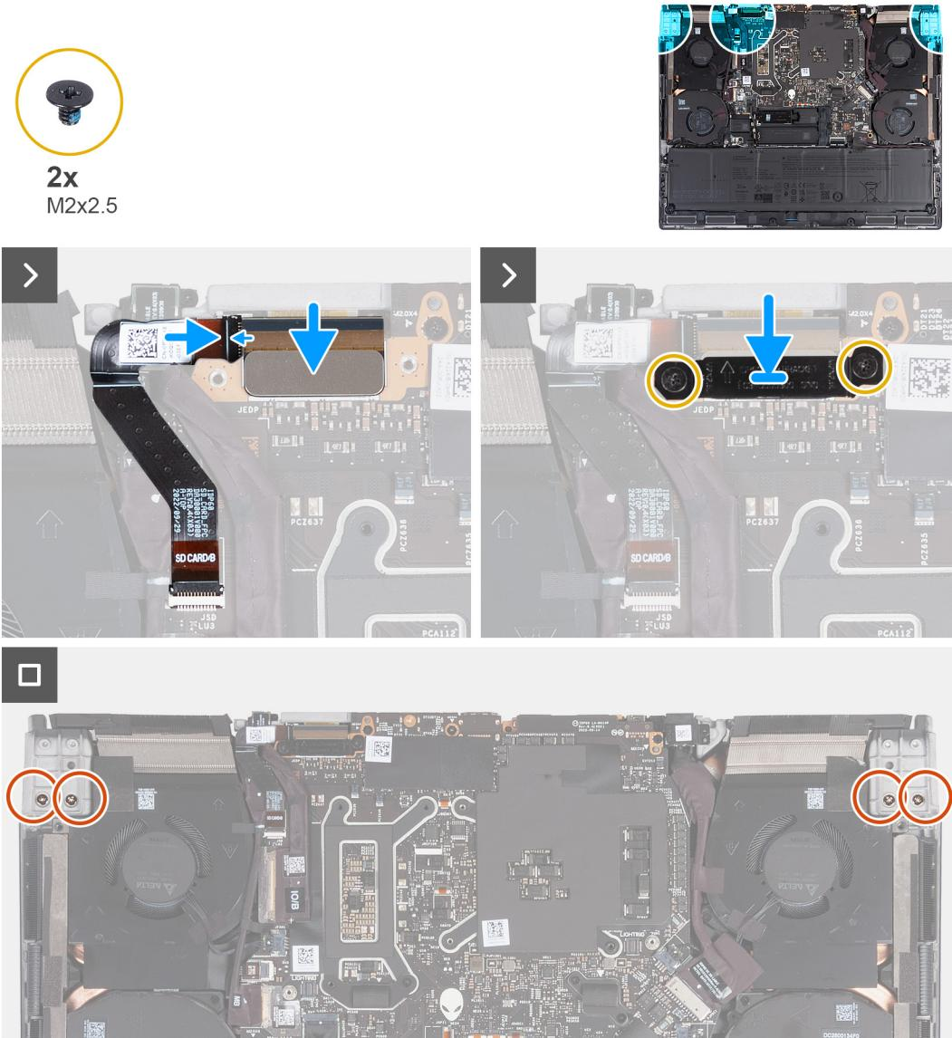
**Figure 57. Installing the display assembly**
