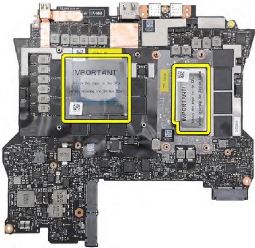
**Figure 72. CPU/GPU Mylar**
