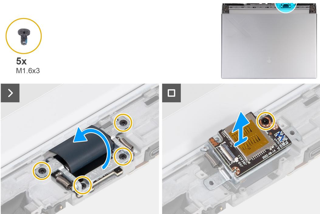
**Figure 45.** Removing the microSD-card reader
