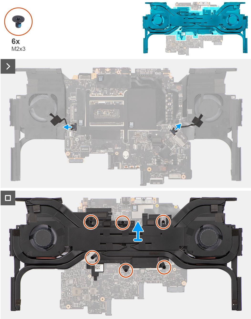
**Figure 78. Removing the fan and heat-sink assembly**
