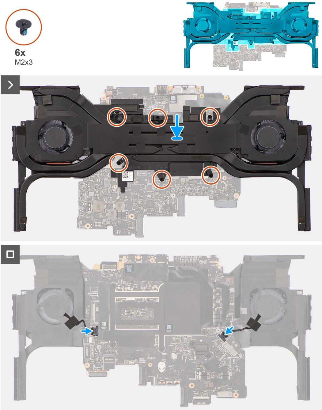
**Figure 79. Installing the fan and heat-sink assembly**
