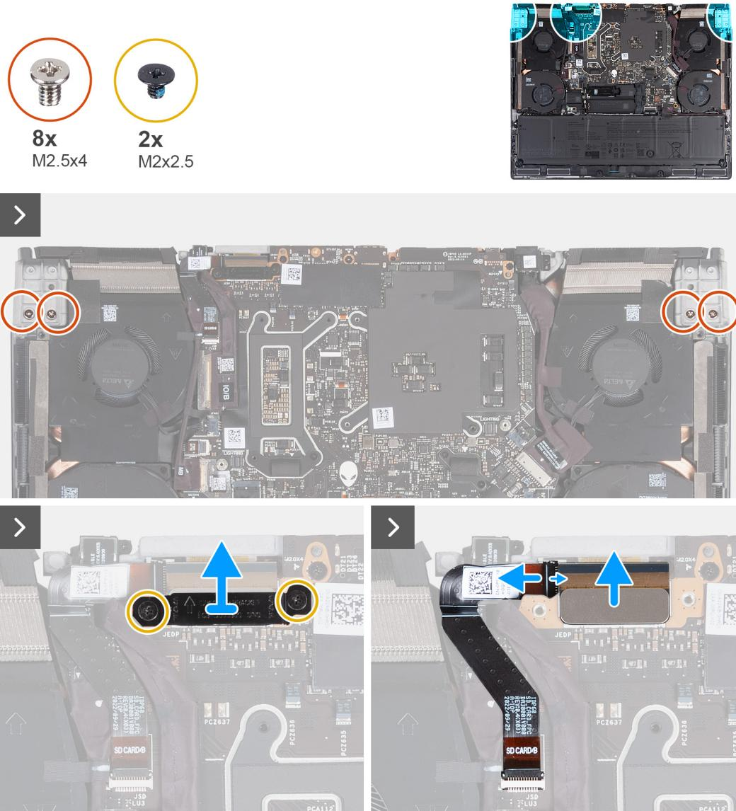
**Figure 50. Removing the display assembly**
