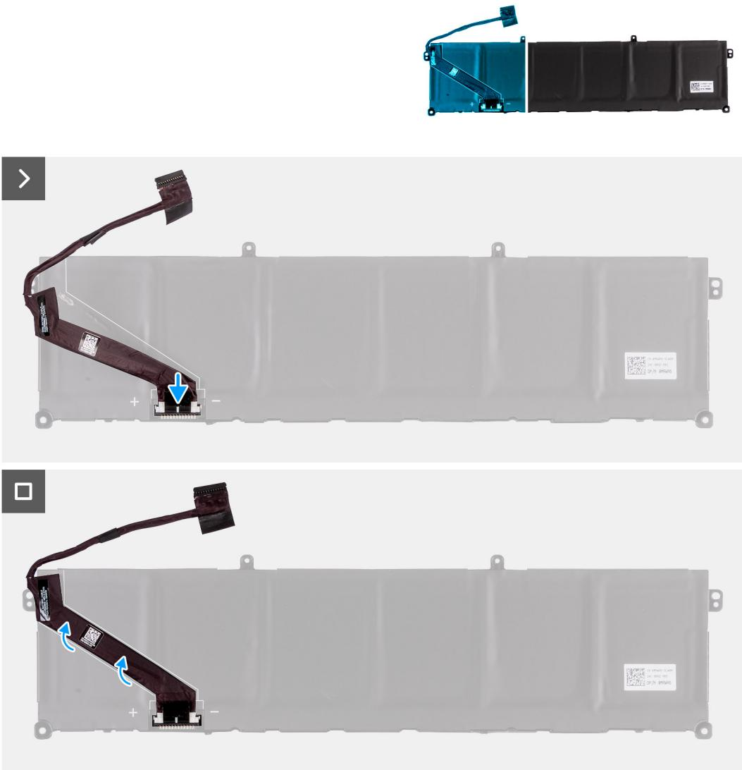
**Figure 34. Installing the battery cable**
