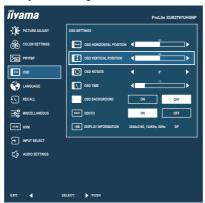
Press the Joystick and finally tilt it [4] to close the On Screen Display feature. All changes are saved in the memory.
