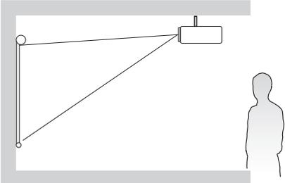
A diagram showing a projector suspended upside-down from the ceiling in front of a screen. The projector is angled downwards to project onto the screen. A person is standing to the right of the screen, looking at the projection. |
