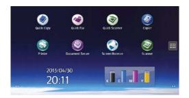
Accessed via a large colour touchscreen display, the smart operation panel is navigated like a smart phone, by tapping, flicking and pinching in/out on the touchscreen. Ricoh's smart operation panel is the most advanced and intuitive available.
