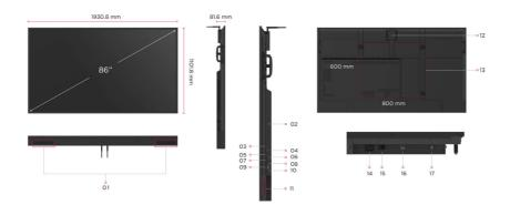
1. Speaker 2. OPS Slot 3. USB 2.0 4. RS-232 5. USB 3.0 6. USB-C 7. HDMI 1(ARC) 8. HDMI 2 9. HDMI OUT 10. HDMI 3 11. Control Panel 12. WiFi Slot 13. VESA® Wall Mount (800x600mm)
