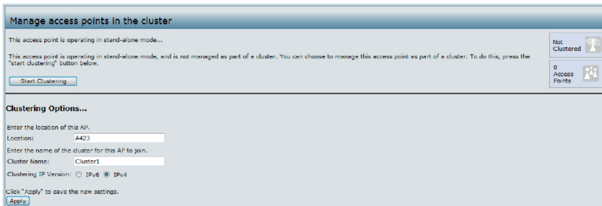
Figure 69 - Manage Access Points In The Cluster (Passive)
