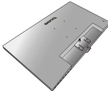
Attach the monitor stand to the monitor base as illustrated until it locks in place.
